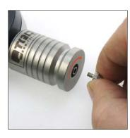
**Step 3**Turn the new tip clockwise until it's stuck.
